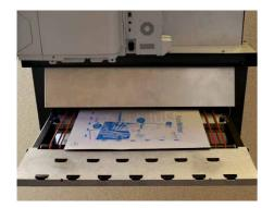
The imaged plates are manually fed through the integrated finishing unit which dries the plates and bonds the liquid dots to the plate surface.
